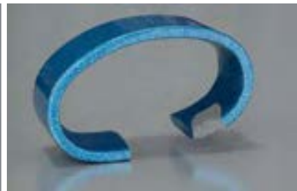
Incorrect Wear Pattern Different Style Required
