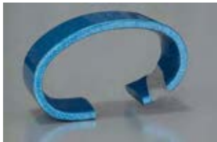
Excessive Wear Pattern Traveler Should Be Changed
